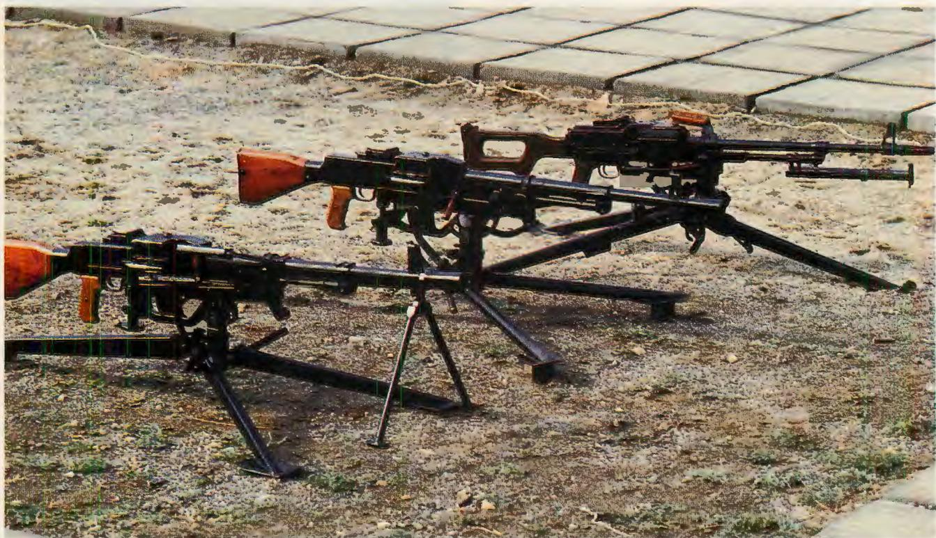
**G**ENERAL Purpose Machine Gun (GPMG). What is it? It's difficult to define precisely. We owe the concept to the Germans and their employment of the MG 34 and MG 42 during World War II. General Purpose Machine Guns are supposed to be capable of serving as both medium machine guns and light squad automatics.
